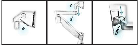
Locate the tilter (e) and insert it into the arm (d). Locate the rail (f) on the back of the tablet and slide the rail (f) onto the tilter (e)
