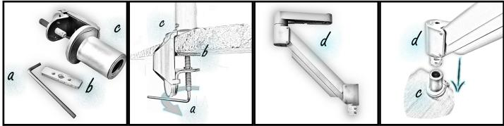
Locate the C-clamp (c), Allen key (a), and base plate (b). Locate a sturdy table edge and tighten the C-clamp (c) by using the provided Allen key (a). Be sure to attach the base plate (b) to the bolt before tightening the C-clamp. down. Locate the arm (d). Slide the arm (d) into the C-clamp (c).
