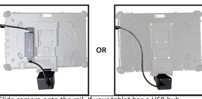
Slide camera onto the rail. If your tablet has a USB hub, connect the tablet to the hub, then the hub to the camera. If there isn't a hub, connect the tablet directly to the camera.
