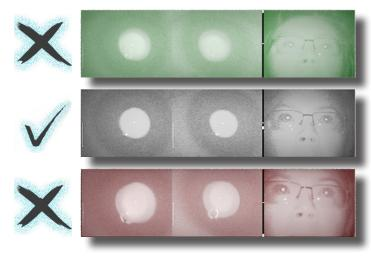
If the eye image is green, the user is too far from the device. The white pin will be somewhere in the upper half of the focus bar. Green means "Go Forward".
